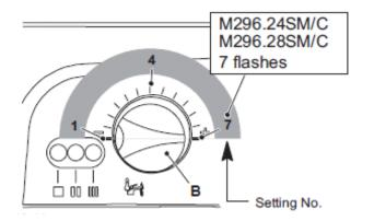
To change the setting, turn the hot water dial (B) to maximum setting 7
