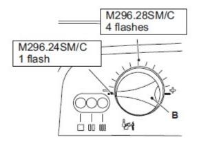
For a **24KW** turn the hot water dial **(B)** to **12 a clock** position and then **turn back** to **minimum** (the lockout lamp **(E)** will start to flash **twice per second**)
